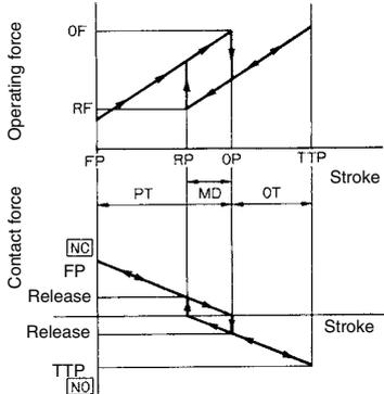
Make sure that the operating body is set so that the actuator should return to the free position when the operating body has moved if a switch is used to form a normally closed (NC) circuit. If a switch is used to form a normally open (NO) circuit, the operating body must move the switch actuator to the distance of 70% to 100% of the rated overtravel (OT) of the switch.
